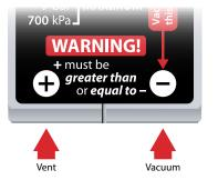
Note: When connected in this orientation, the XP2i-DP display will invert the sign on the gauge display. For example, a pressure of -12 psi on the negative port will display +12 psi. To invert the sign to read -12 psi, use ConfigXP Software (V 2.4 or later).
